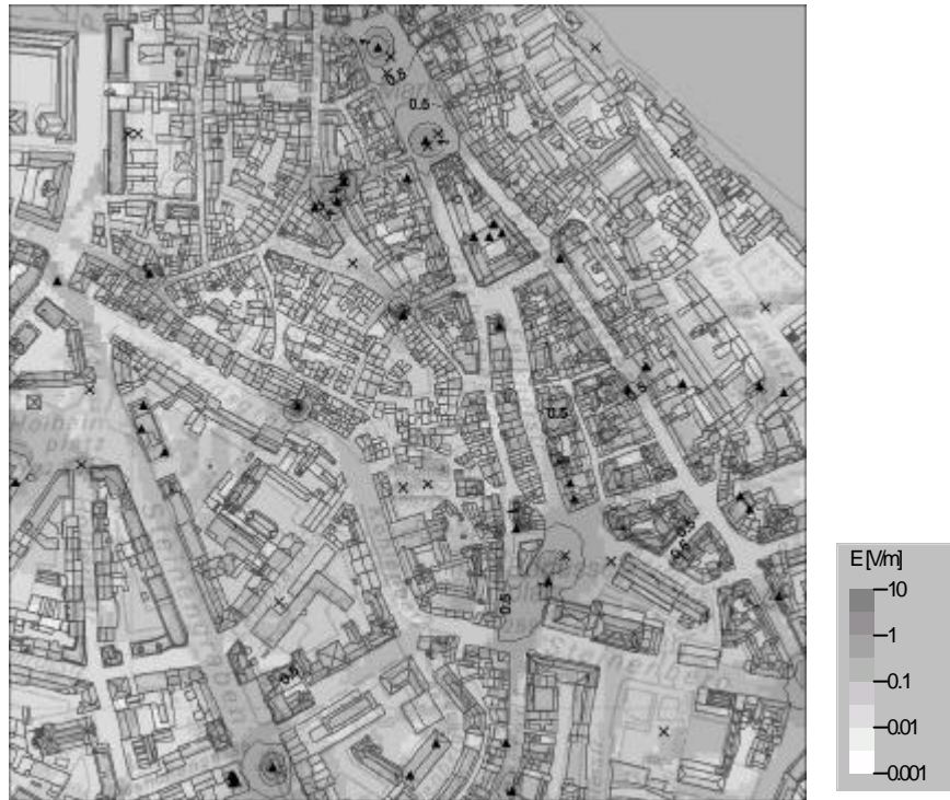
Figure 3: Black-and white approximation of the map of the electric field superimposed on the city map for model region B (centre of the old city of Basel). The equidistance of the contour lines is 0.5 V/m. The Rhine river is in the upper right corner. Basel city model used with permission of 7.12.2004, © Office of land register and surveying, Basel.
